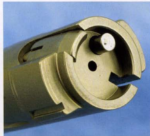
The slightly fatter than normal bolt provides extra wall thickness for the recessed bolt face. Note the plunger ejector and the slot in the bolt head for the static ejector, giving the G30 two separate ejection systems.
