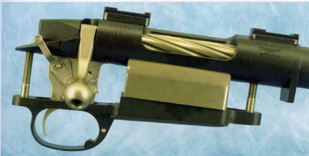
The G30 action is quite conventional in that it employs a tubular receiver and separate recoil lug. The magazine box is fabricated sheet metal that engages skirts in the receiver and bottom metal unit.
