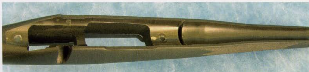
The EDGE graphite stock weighs only 24 ounces but is extremely rigid. The G30 action is beautifully glass bedded; the barrel, however, is fully floated the entire length of the fore-end.
